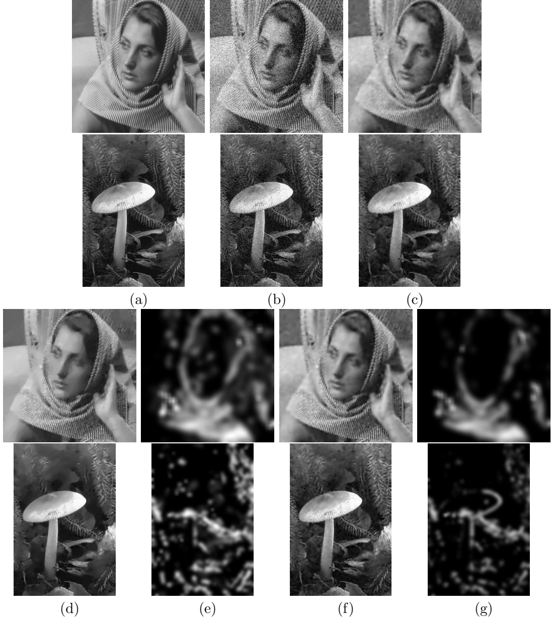
FIGURE 1. Example 1: Comparison of 10% Gaussian noise removal. (a) The original images, (b) the noisy images, (c) results of the TGV method with \lambda = 10 (row 1: PSNR=25.69 dB; row 2: PSNR=27.39 dB), (d) results of the SA-TV method (row 1: PSNR=26.39 dB; row 2: PSNR=27.12 dB), (e) final values of \lambda by the SA-TV method, (f) results of the SA-TGV method (row 1: PSNR=26.83 dB; row 2: PSNR=27.53 dB), (g) final values of \lambda by the SA-TGV method.
